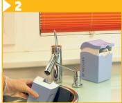
Fill container with cold water up to the indicator (= 600 ml of 1% dilution)
