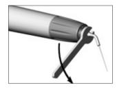
• Unscrew the tip using the spanner.
