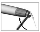
2 Screw the tip down using the spanner.
